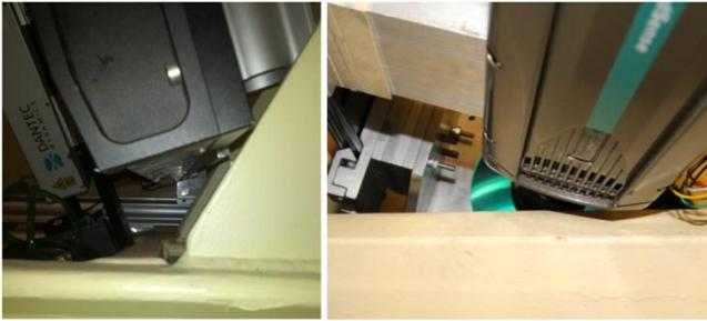
**Figure 9:** Tilting limitations due to ship's frame construction at porthole 2 (right); disturbing toe bracket for rotation around Y (left).
