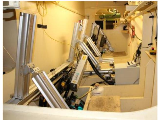
**Figure 4:** Measurement setup inside the steering gear compartment.
