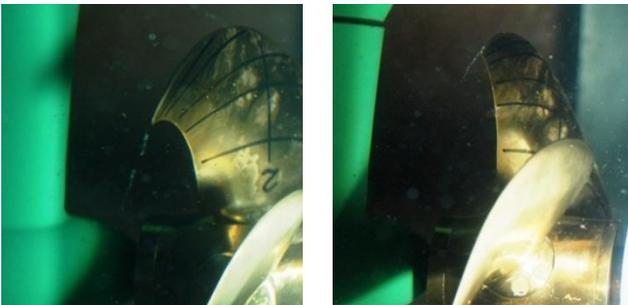
**Figure 19:** Tip vortex cavitation on the model propeller in the operation point.
