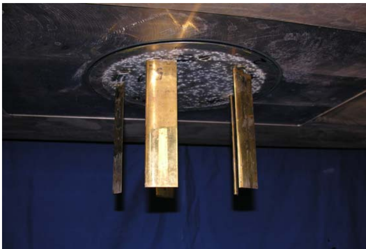
Fig. 14 Rotor casing with VSP blades P9659_R in the cavitation tunnel
