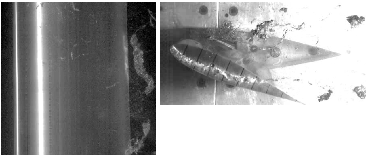
Fig. 8 Cavitation observation, angle of attack = 12^\circ , V_M = 4.00 m/s, \sigma_V = 2.40
