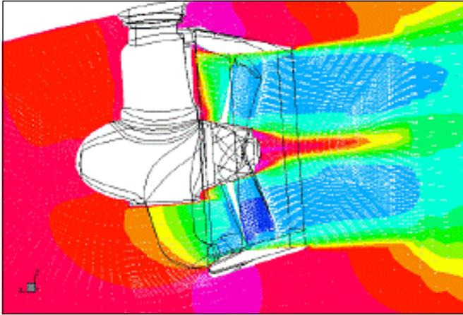
Figure 1: Axial velocity components in a longitudinal section of an SRP.
