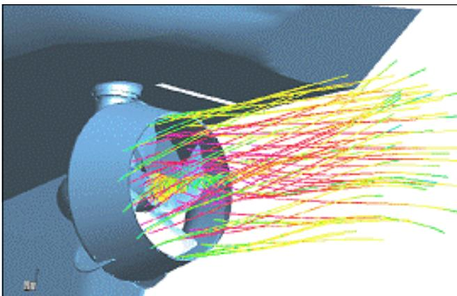
Figure 2: Stream lines in the propeller jet.
