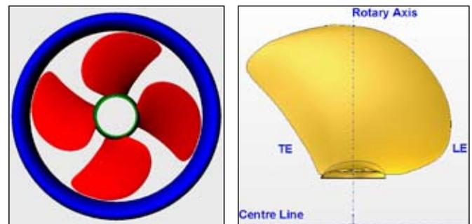
Figure 13: Propeller VP 1466 in nozzle and 3D model of full-scale propeller ( $D_p = 4.40\text{m}$ ).
