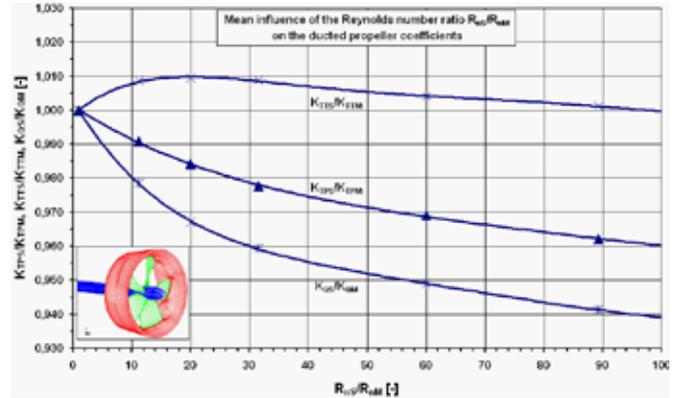
Figure 4: Influence of the Reynolds number ratio on the change of the ducted propeller coefficients.
