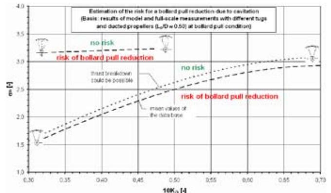
Figure 10: Estimation of the risk of bollard pull reduction due to cavitation.
