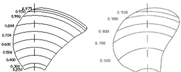
Figure 5a: Blade outlines – left, Kaplan blade shape VP 1303; right, diminishing chord length at the blade tip VP 1305A.
