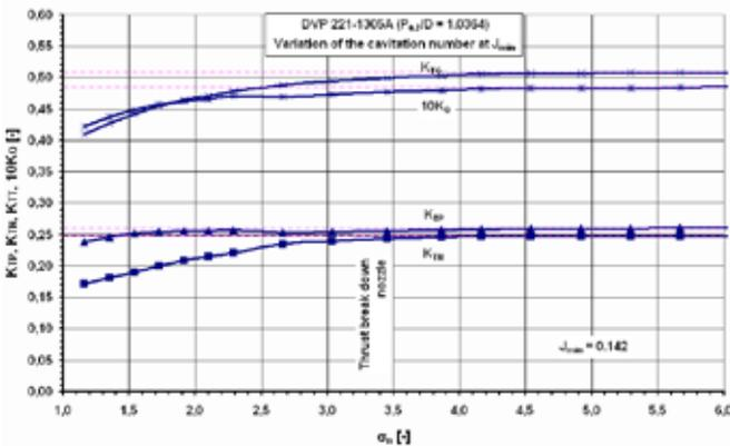
Figure 7: Variation of the cavitation number, DVP 221-1305A.
