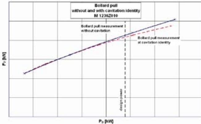
*Figure 17: Bollard pull without and with cavitation identity, M1236Z010.*
