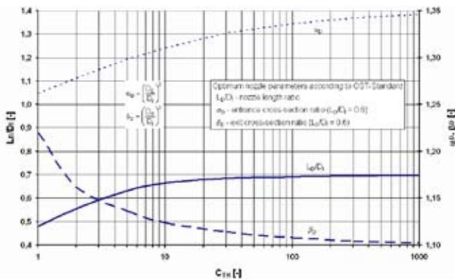
Figure 12: Optimum nozzle parameters (OST Standard<sup>8</sup>).
