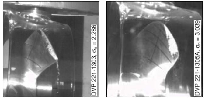
Figure 8: Cavitation behaviour at the cavitation number for the inception of nozzle thrust breakdown.
