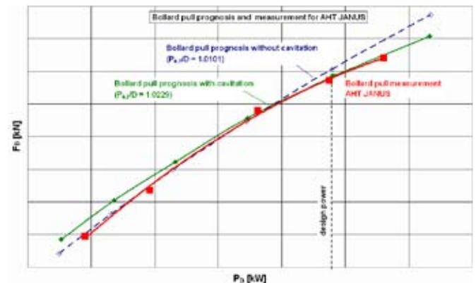
*Figure 21: 220 T AHT Tug JANUS, comparison of bollard pull prognosis and measurement.*
