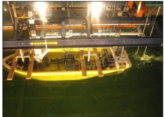
Figure 16a: Model M1236Z010 in the test section of the UT2.
