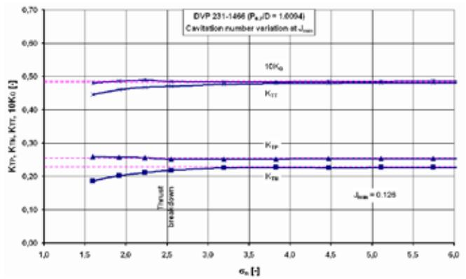
Figure 15: Variation of the cavitation number, DVP 231-1466, first propeller design.
