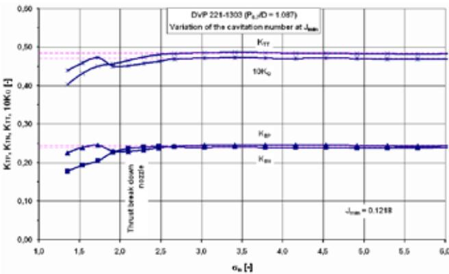
Figure 6: Variation of the cavitation number, DVP 221-1303.
