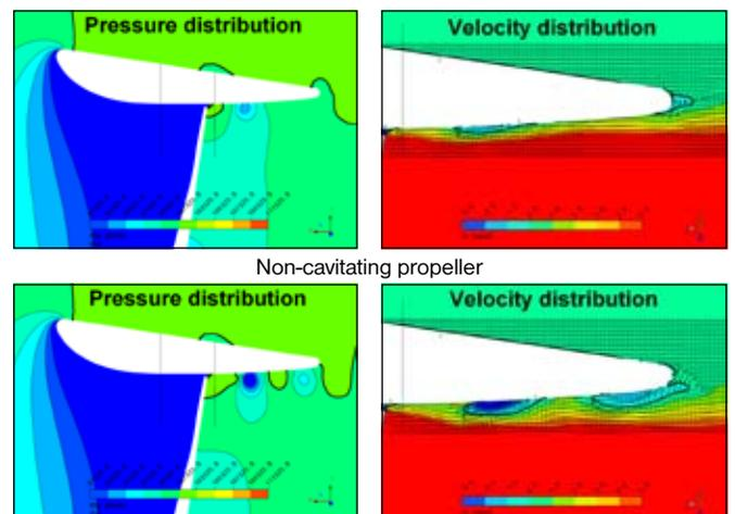
Cavitating propeller, inception point for thrust breakdown
