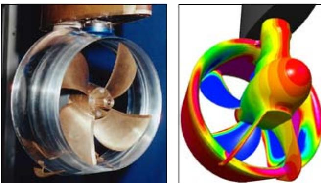
Figure 3: SRP in model test and CFD calculation (pressure distribution).
