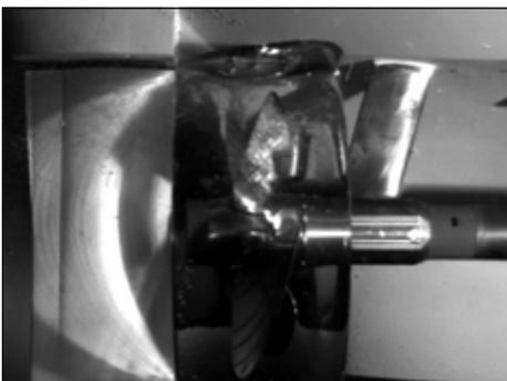
*Figure 18: Cavitation observation model M1236Z010,  $\sigma_n = 2.60$  (cavitation identity).*
