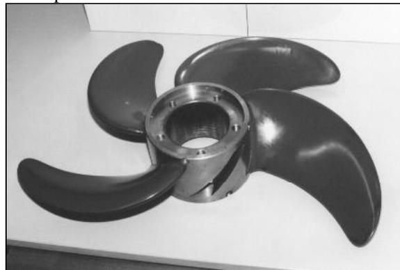
Figure 20 - 5 bladed model of the CONTOUR (F) single rotor propeller (Carbon fibre reinforced material).
