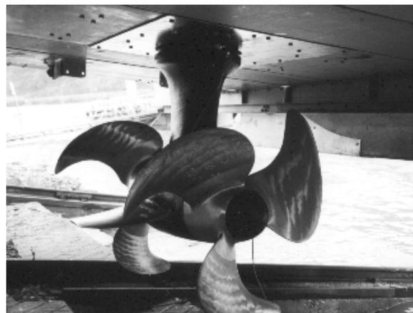
Figure 18 - Test arrangement of a SCHOTTEL-TWIN Propeller
