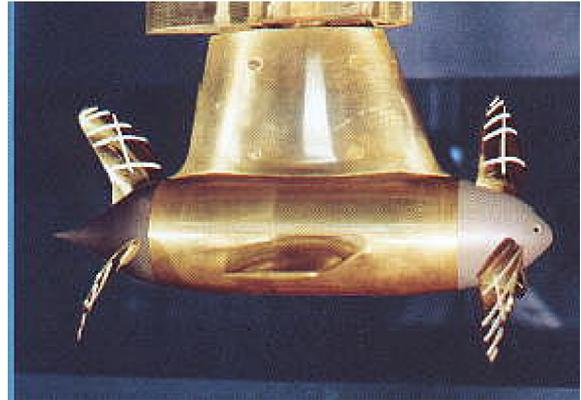
Figure 8 - SSP 7 TWIN-Propeller as PoD-Propeller (test model in the SVA cavitation tunnel)
