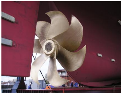
Propeller for FRV SOLEA designed for low noises
