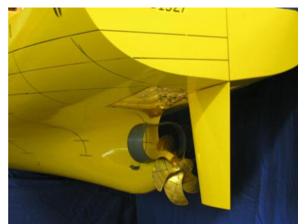
Schneekluth nozzle in model test
