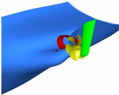
ship with wake equalizing duct
