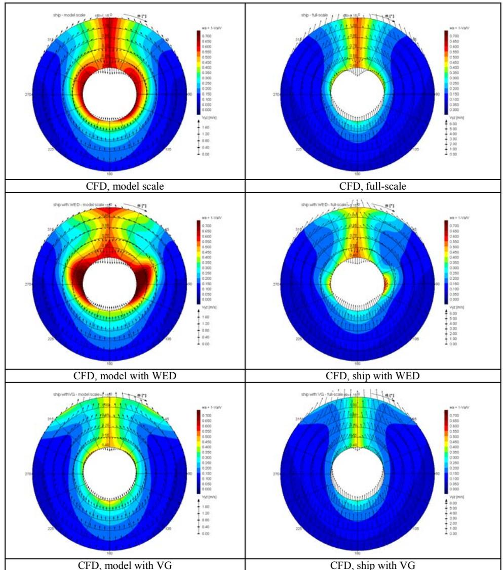
Figure 2: Influence of the Reynolds number on the propeller inflow of a container ship
