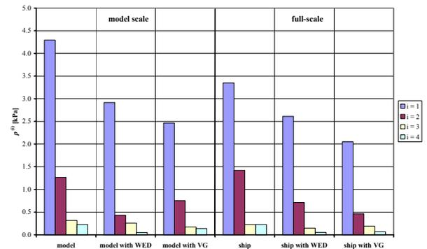
Figure 3: Pressure fluctuation amplitudes, propeller in the calculated model and full-scale wake fields
