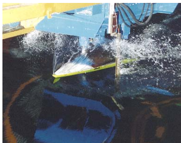
Slamming test in a wave packet, V = 6 m/s
