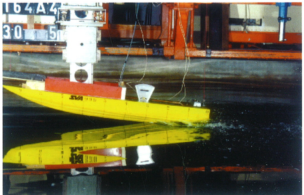
Seakeeping test with a model of a patrol boat V = 45 kn, \lambda/L = 3.0
