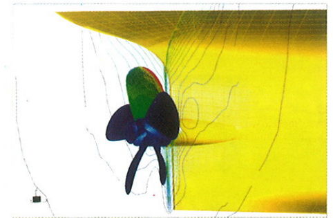
Calculated unsteady propeller inflow
