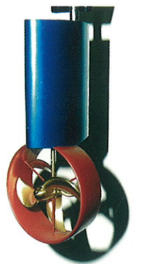
Contrarotating propeller-nozzle thruster
