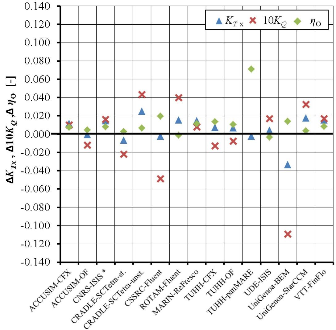
**1.23 Absolute difference between measured and calculated values:  $\psi^P = 12^\circ, J = 1.0$**
