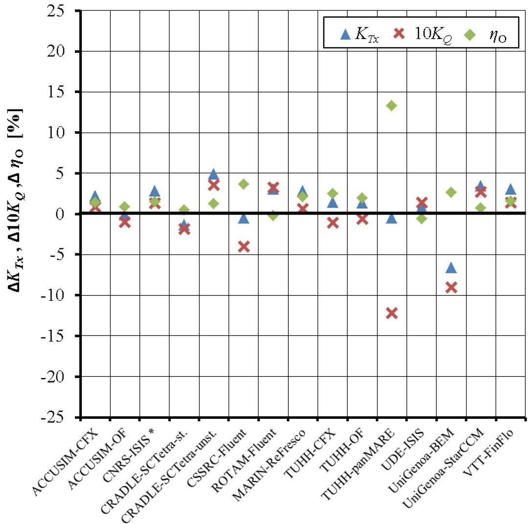
1.28 Relative difference between measured and calculated values:  $\psi^P = 12^\circ, J = 1.0$
