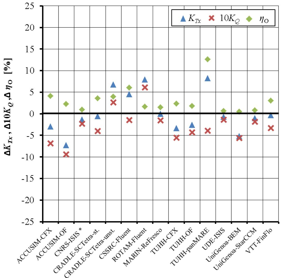
1.30 Relative difference between measured and calculated values:  $\psi^p = 12^\circ, J = 1.4$
