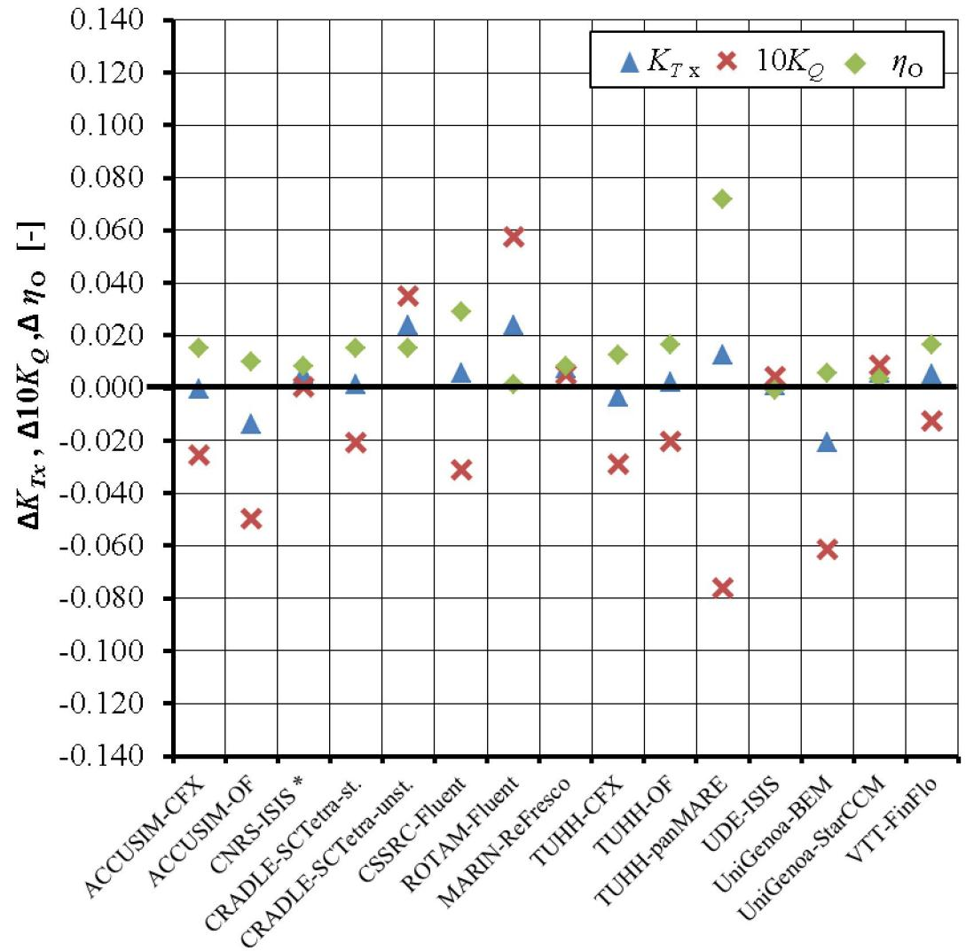
**1.24 Absolute difference between measured and calculated values:  $\psi^P = 12^\circ, J = 1.2$**
