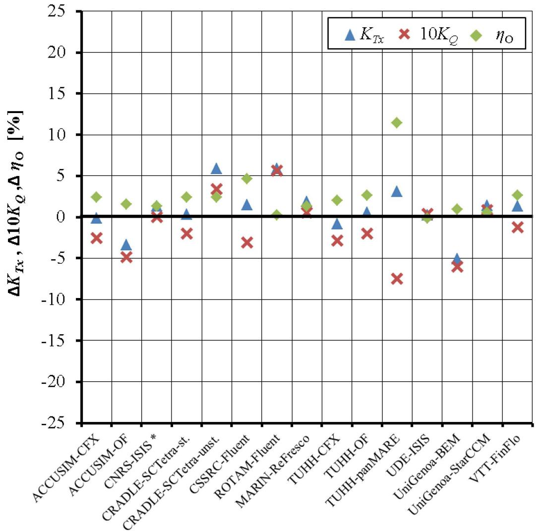
**1.29 Relative difference between measured and calculated values:  $\psi^p = 12^\circ, J = 1.2$**
