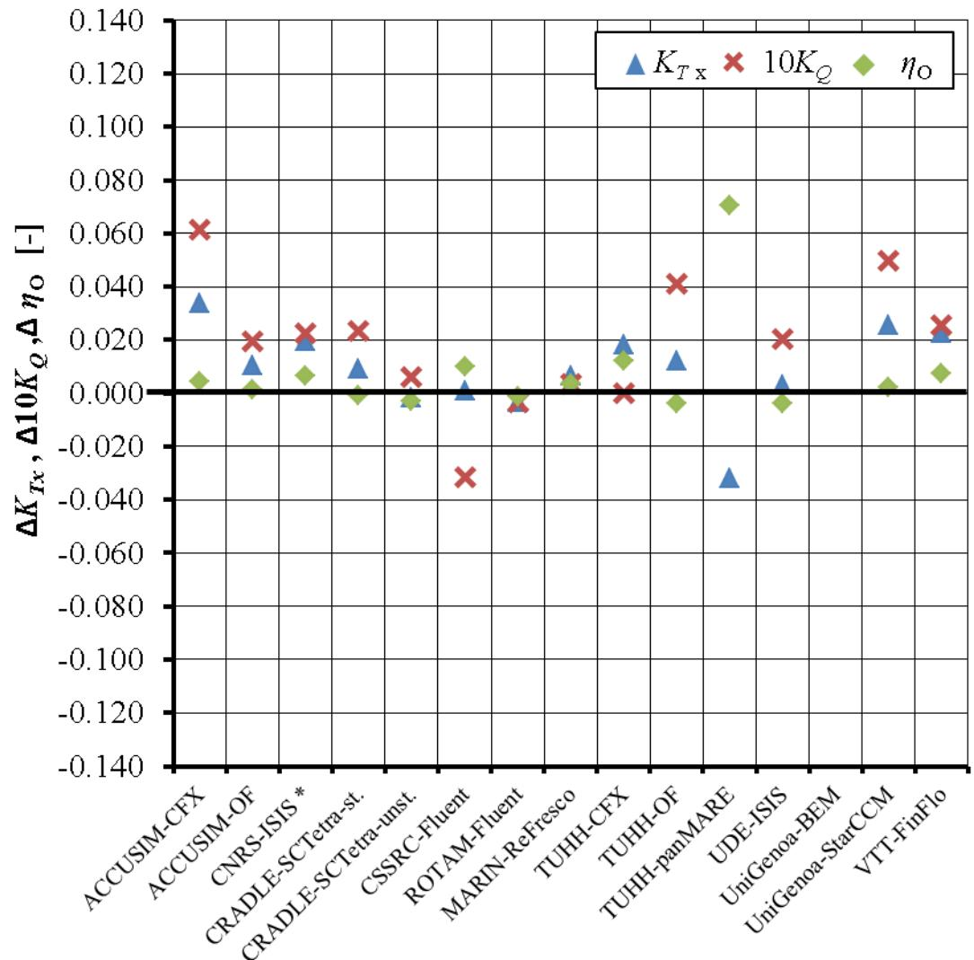
**1.22 Absolute difference between measured and calculated values:  $\psi^P = 12^\circ, J = 0.8$**
