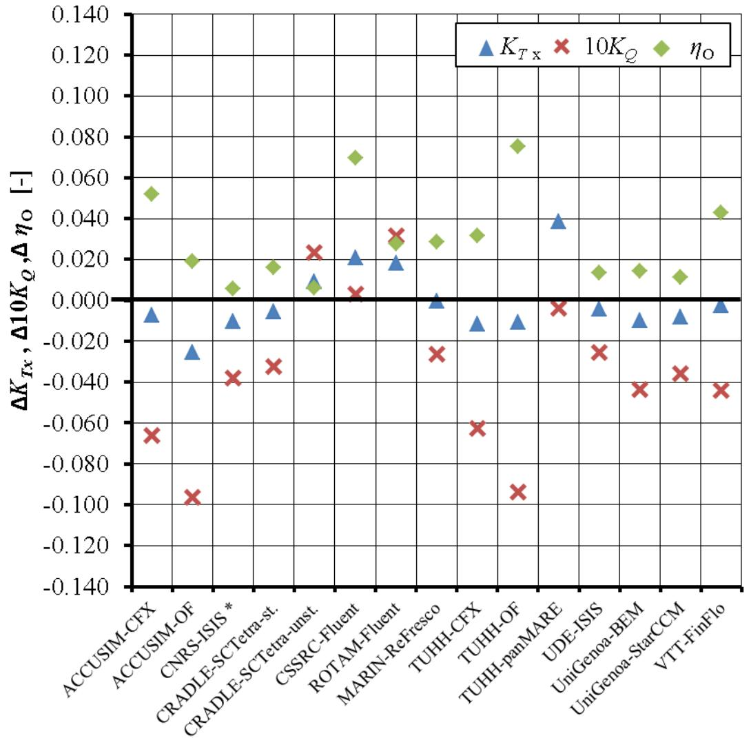
**1.26 Relative difference between measured and calculated values:  $\psi^p = 12^\circ, J = 0.6$**
