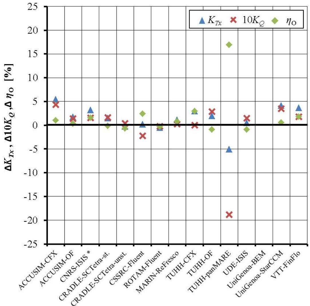
**1.27 Relative difference between measured and calculated values:  $\psi^p = 12^\circ, J = 0.8$**
