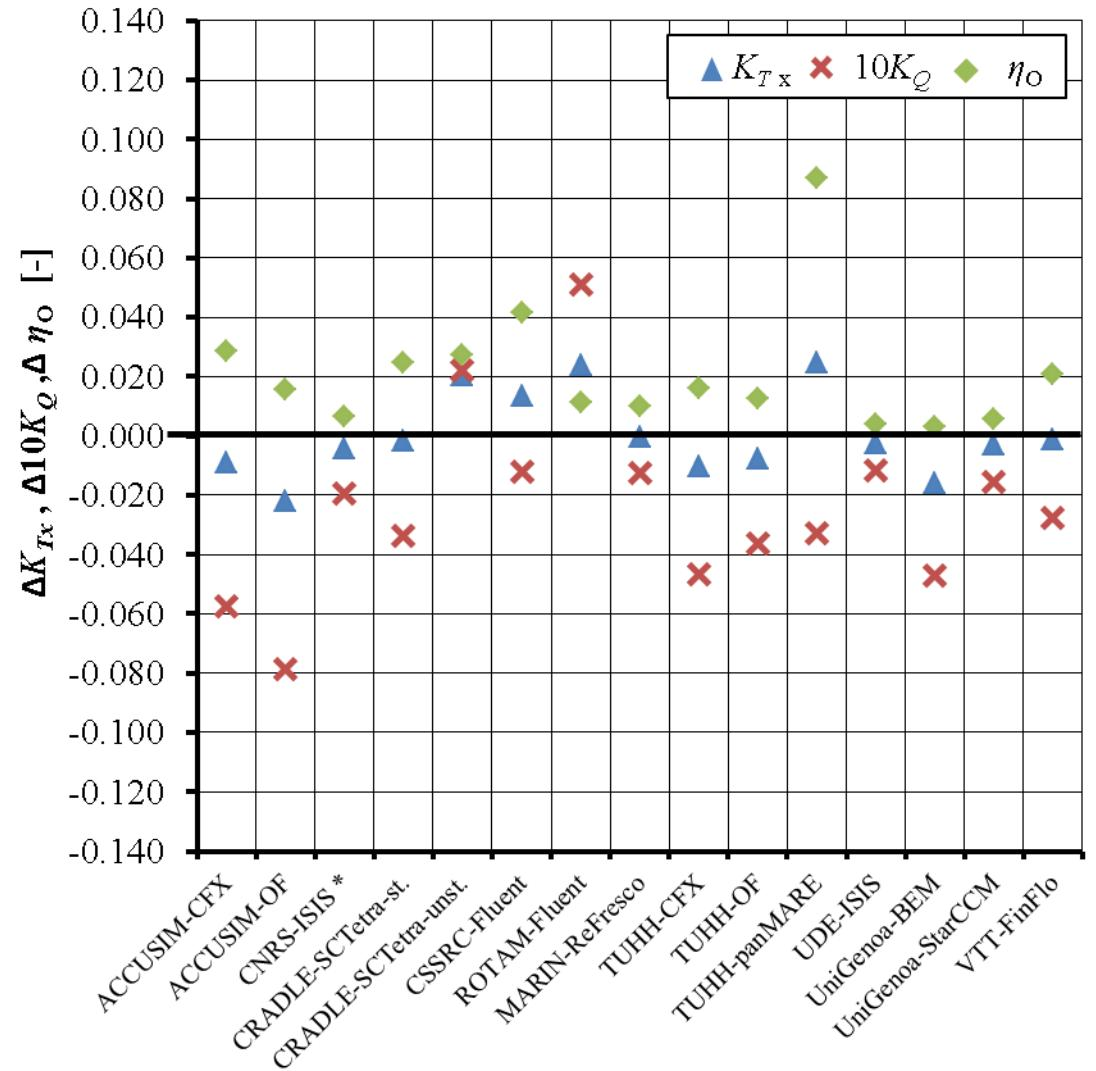
**1.25 Absolute difference between measured and calculated values:  $\psi^P = 12^\circ, J = 1.4$**
