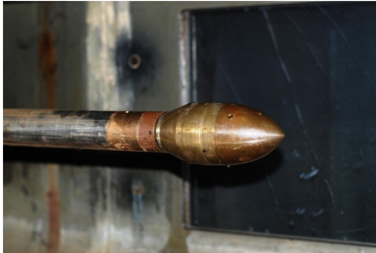
Measurement of idle torque with a dummy hub
