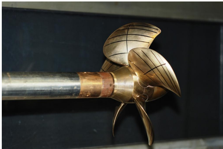
Measurement of idle torque with a dummy hub
