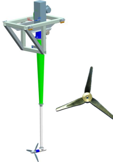
Test set-up for turbine rotors
