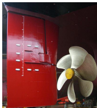
Full-scale measurements, ship with semi-balanced rudder
