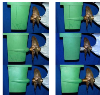
Systematic variation of boss caps, rudder bulbs and rudder-propeller distances
