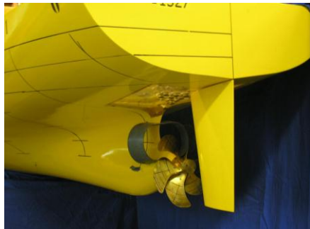
Ship model with Schneekluth nozzle
