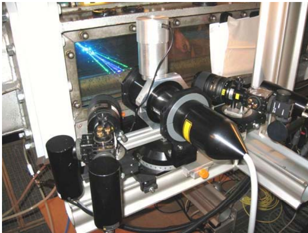
Figure 7: Experimental setup at K21. center: LDA transmitter, TST laser diode and light sheet generation, left and right: adjustable receiver optics with dichroic and polarization beam splitter and two photomultipliers each side.
